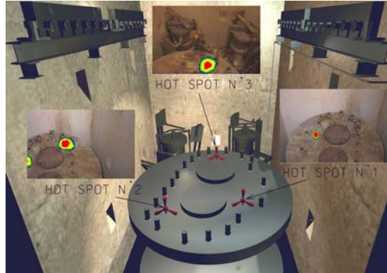
Figure 6: 3d As-Built CAD Model with hot spot representation
